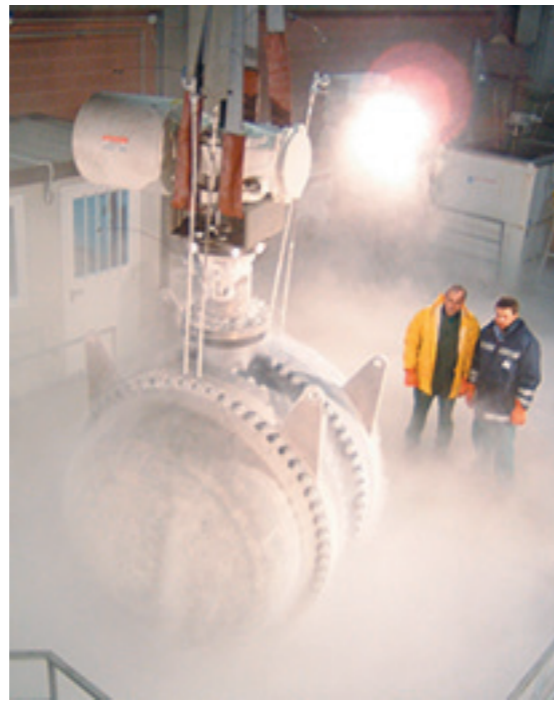
66" cl. 150 actuated after cryo test
